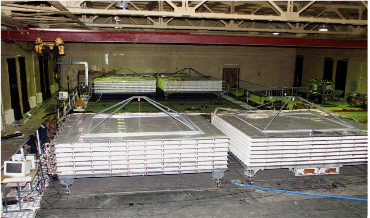
Hodoscope - instrument that traces the path of a charged particle
