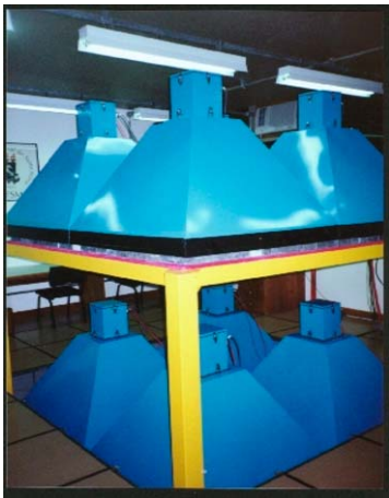
Figure 2. The prototype muon detector installed at SSO.
