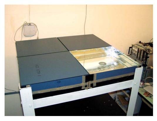
pic. 1. The cherenkov detectors from the upper plane during assembling.
