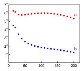
Fig. 3. Variation of the median angle, (a)  $\alpha_{mp}$  for plane fit shown by filled circles , (b)  $\alpha_{mc}$  for cone fit shown by filled squares, as a function of number of hit detectors .
